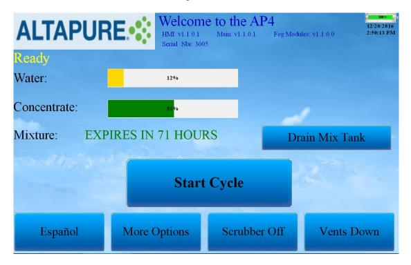
5. If the Water or Concentrate show low (yellow bar) you will need to fill it prior to starting a cycle. To add water, remove the black cap labeled "WATER ONLY". Fill with reverse osmosis (RO) and/or deionized (DI) water until the display shows close to 100%. Add 1 mL of Altacare concentrate per gallon of water to assure freshness. Make sure to add some water after the concentrate is added to rinse it down the filler tube. Do not use tap water or filtered drinking water. Replace the cap.
